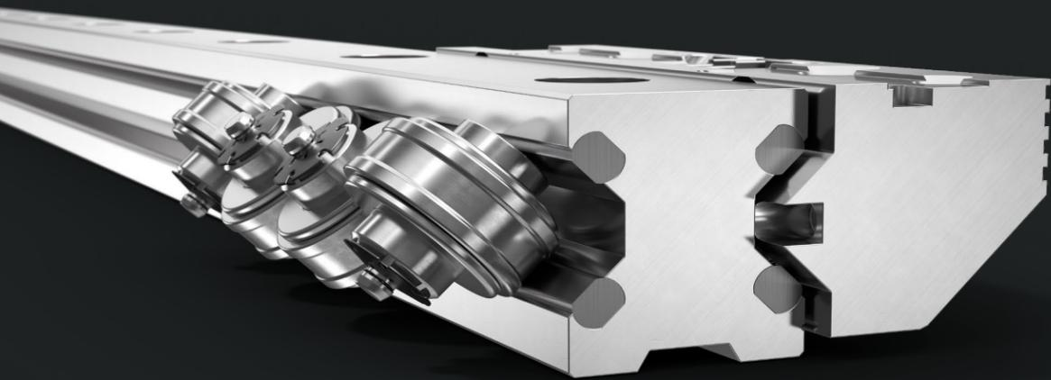
Franke linear guides are the first choice when highest dynamics are required. The large rollers are mounted very smoothly. They run with low friction and precisely guided on the inserted tough and hard steel wires. Because almost exclusively light aluminum is used for the entire construction, the moving mass is low. The result: Highest dynamics and energy efficiency.
